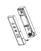
FIG. 2 - BATTERY PLACEMENT
